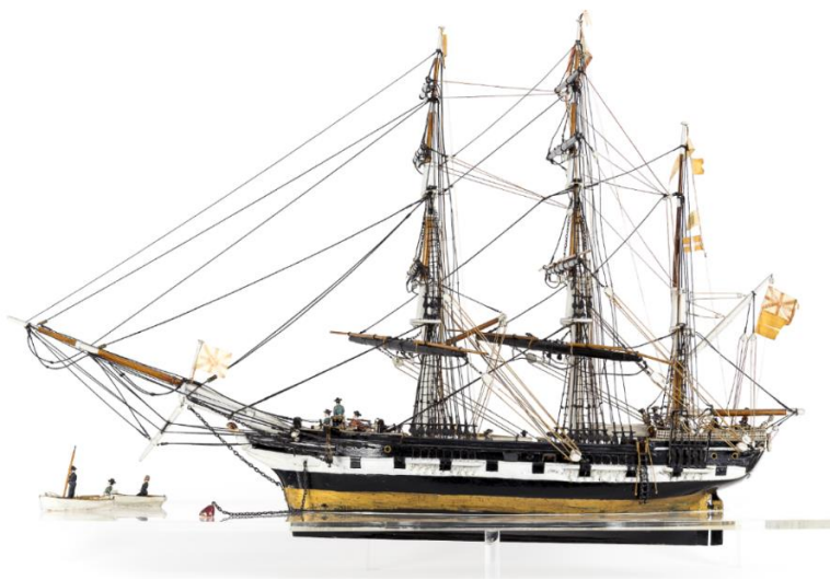
The Philip Laing , model made by crewman Henry Godfrey. Otago Museum. The Amelia Thompson came from the same shipyard and with her long (43 ft) bowsprit and 40ft jib boom would have looked similar when she was barque rigged.
