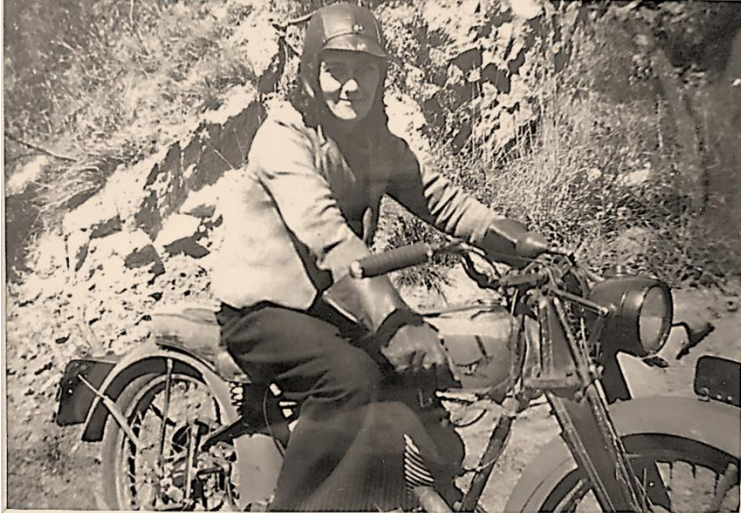
Eleanor Pearl Stokes on a Wolf Vixen motorcycle, Central Otago, about 1930. The Vixen had a 148cc Villiers twin port engine with a 3 speed hand change Burman gearbox. She has her right hand on the gear lever.
